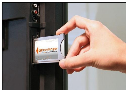
The Module inserted in the CI Plus Interface of a flat TV
